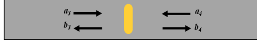
Fig. 3. The portion of the hybrid structure in Fig. 2 consisting of the plasmonic nanoresonator is modeled as a hybrid waveguide-based structure, which is excited from both ends.
